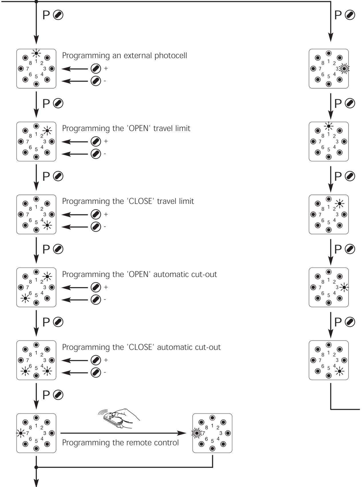
The programm is stored by pressing programming button P and the programming process is completed; recognizable by running light through all the indicators. The control unit is now in the operating state.
