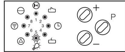
The operator allows connection of an external signal light, provided the relay retrofit kit 'OPEN-CLOSE+light door function' for standard operators in a housing (item no. 152 137) is connected and the automatic timer is activated. The output can be programmed in such a way that the signal lights flash or glow.
