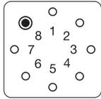
Operating state (indicator 8 glows; if the door is in an open or closed state, the corresponding indicators 2 or 4 also glow).
